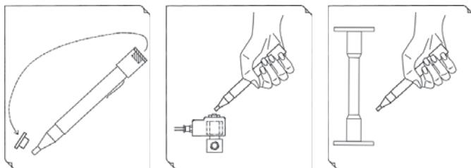
*MasterEx 79504 is a pen-sized magnet probe, designed to detect magnetic fields in hazardous areas. Within seconds it is possible to detect whether or not a solenoid valve is electrically activated.*
