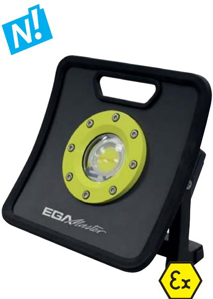
The MasterEx 79732 and 79733 hand lamps are specially designed to (illuminate) light large spaces in hazardous areas. The two LED modes (50% and 100% output) allow to adapt the intensity of the emitted light. The lamps are suitable for use in zones 1 and 21.
