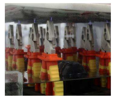
Our insulated tools follow the verification process indicated above, and therefore meet the requirements indicated by the international standard IEC 60900. These offers:
